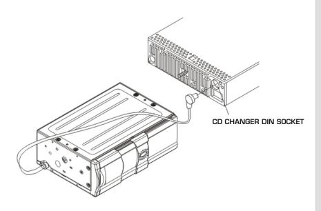
When you want to play the CD changer, plug the CD changer DIN into the socket of the back of the car audio unit.
